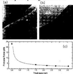
force was much weaker than the attractive force. Figure 1 shows representative topographic (a) and LFM (b) images of multi-layers of graphene measured simultaneously with a SiN cantilever in air. (c) The frictional forces were measured as a function of the thickness of the graphite film.
