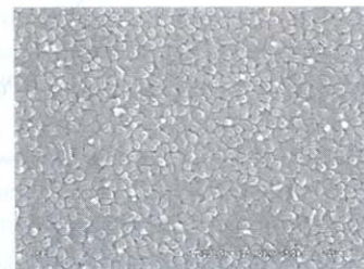
Figure 2. SEM image of Cu-Pc thin film at the room temperature.
